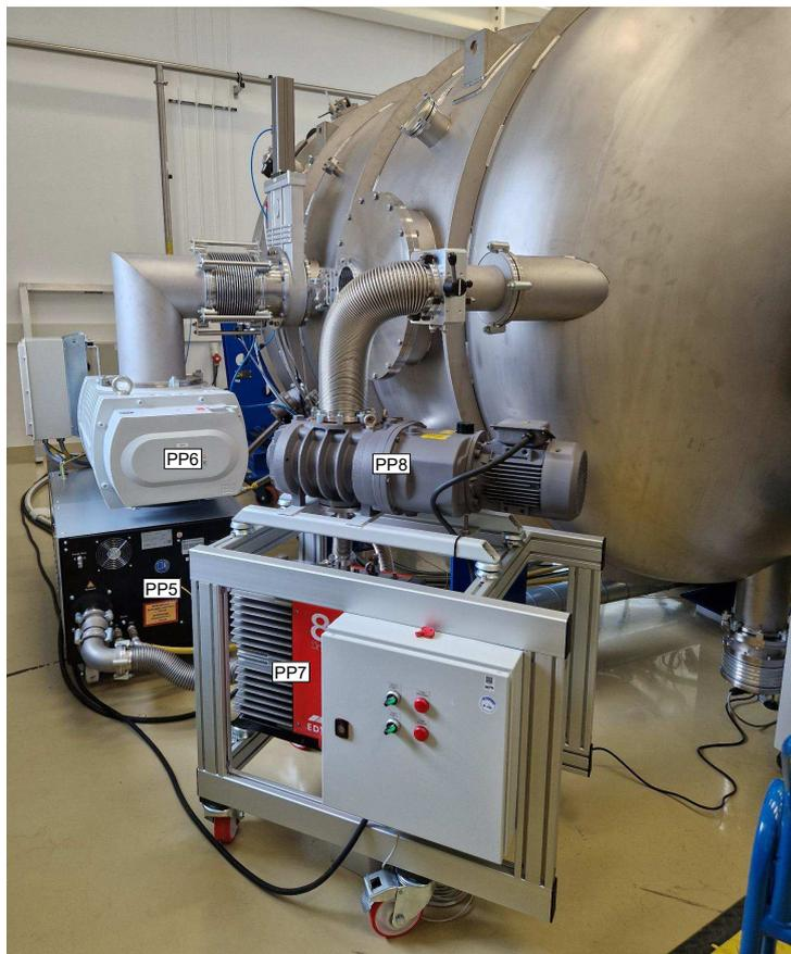
**Figure 4.5.:** Primary pumps on the SPF used in this test (PP5,PP6 and PP7,PP8)
