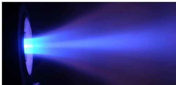
**Figure 2.7.:** Operational Magneto-Plasma-Dynamic Thruster (SX3, University Stuttgart) [8]
