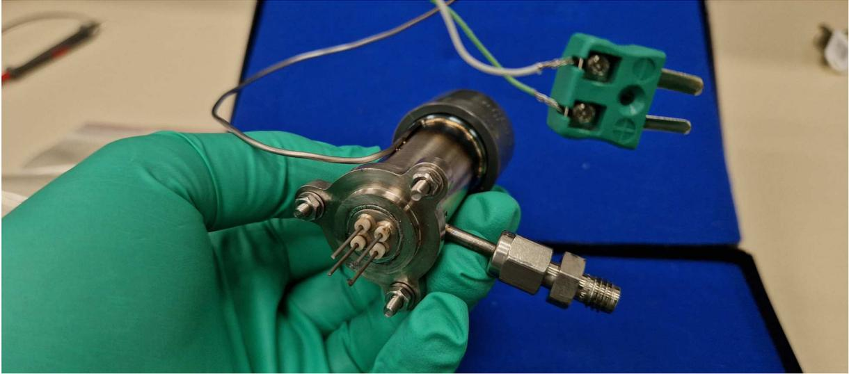
**Figure 4.2.:** The XR100 resistojet in the ESA propulsion laboratory
