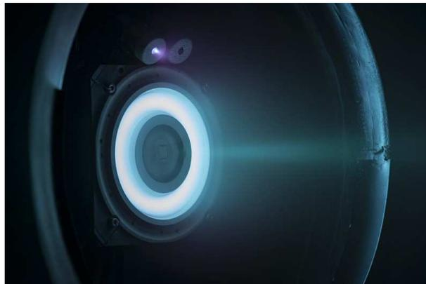
**Figure 2.3.:** Operational Hall Effect Thruster (PPS-1350G, Safran Aircraft Engines) [11] Originally CNES, 2015
